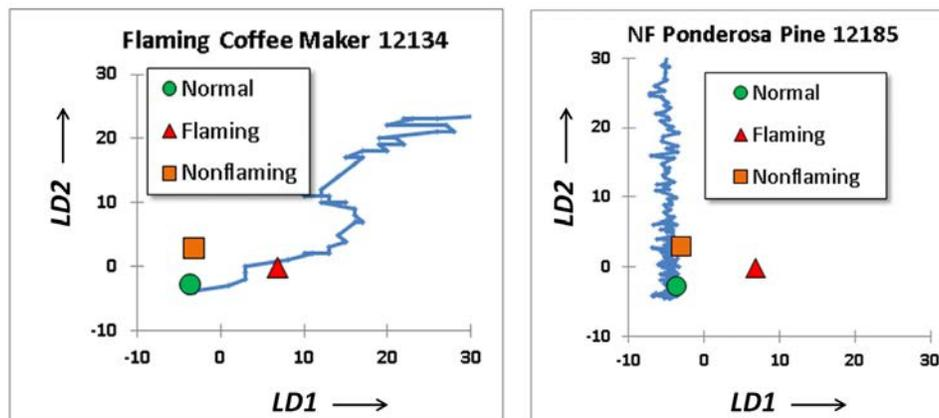
Figure 1. Illustrations of the LDA coordinate progression in an example of flaming fire (left) and nonflaming or smoldering fire (right). The LDA centroids of the test conditions of normal, flaming and nonflaming are indicated.
