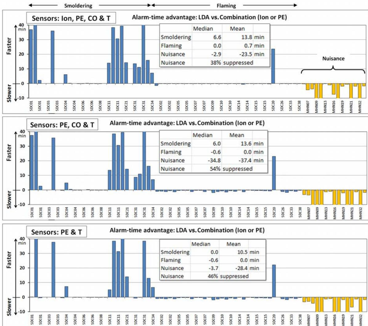
Figure 3. Comparison of alarm times for various LDA-based sensor sets against a combination alarm with an ionization and photoelectric sensor in which the most sensitive setting is used for both sensors. The bars represent individual tests segregated according to flaming, smoldering and nuisance situations. The median and mean times to alarm for the LDA algorithm are given in the insets.
