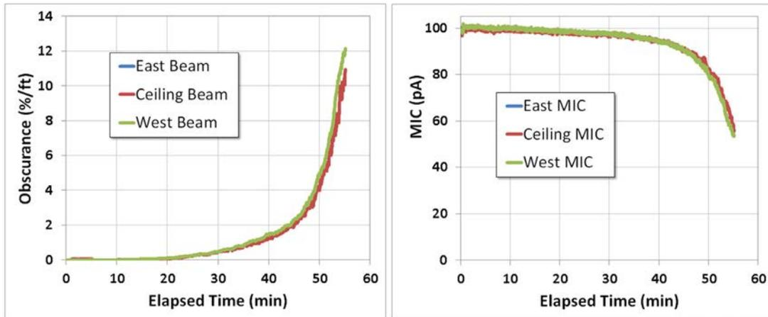
Figure 5. Lamp obscuration and MIC reading during Test 15 – Smoldering Wood.
