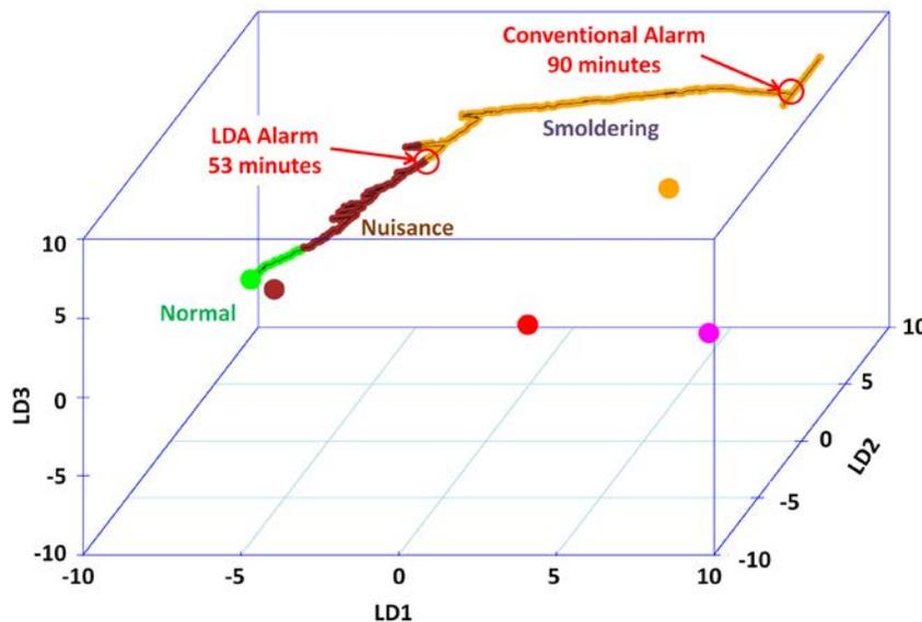
Figure 2. Progression in three dimensions of LD space for data recorded by NIST<sup>16</sup> during a smoldering chair test (SDC01A). Conditions are color coded: Normal (green), Nuisance (dark brown), and Smoldering (light brown). The colored circles represent the centroids of various fire conditions.
